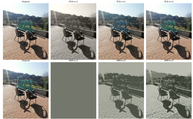
Fig. 11. Clustering results with k = 1, 2, 3 corresponding to PCA dimensions on a real photograph.
